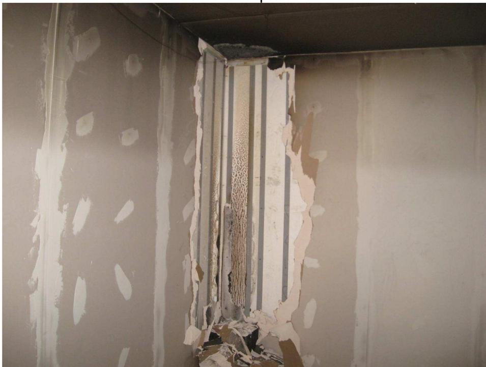
Post-test photo with Gypsum removed form corner
